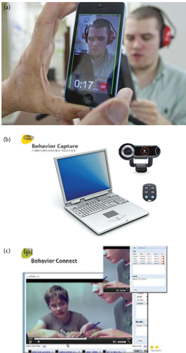
Figure 17.1 Illustration of the key components of the new technology platform: (a) App options to enable video capture for smartphones, (b) laptops, and (c) associated online clinical assessment interface.
