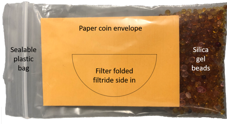
Figure 3. A filter membrane is folded in half with the filtride side in and placed inside a paper coin envelope. This, in turn, is placed in a sealable plastic bag containing silica gel beads, the air removed and firmly sealed before storage. It is easy to monitor the moisture content of the sample. The orange beads turn dark green when there is too much moisture and need to be replaced or the beads regenerated as per the manufacturer's instructions.
